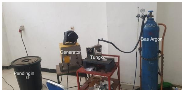
Gambar 2. Setup Peleburan EAF
